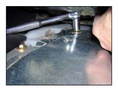
You may choose to remove 2 screws (1 on each side) that are located close to the new mounting holes that are required. The photograph above shows the carpet and padding lifted and the left side screw being removed adjacent to one of the new holes.
