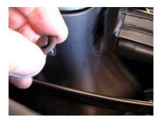
Carefully lift the center pin using a sharp tool and pull out the fastening clip as shown.
