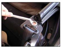
Remove the plastic cover and large 17mm bolt from the top of the "B" pillar.
