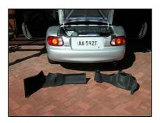
Remove the split trim panels by unclipping the appropriate plastic fasteners.
