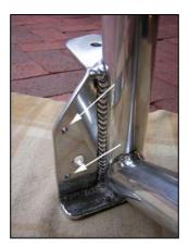
Drill and tap 4 holes (to suit 6mm screws), to suit fabricated brackets such as those shown next.
