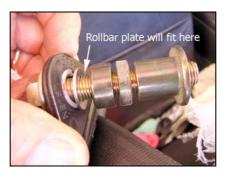
Remove the spacer that is approximately 7mm thick - it will not be required during reassembly. It will be replaced by a suitable spacer (1, 2 or 3 washers – depending on washer thickness) that will allow freedom for the support bracket to pivot and also sufficient height for the plastic cover to be refitted later. Note the 3 tabs on the plastic cover as shown above.
