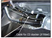
Remove the inner metal panel that covers the petrol fittings. Relocate the CD stacker cable if needed. DO NOT allow it to be sandwiched between the roll bar flat plate and the rear parcel deck.
