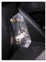
These photographs show the new bracket in place. Note the large hole that was punched prior to folding the bracket. It allows clearance of the fixing bolt that fastens the roll bar to the "B" pillar (see Step 9 below).
