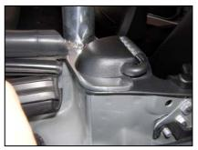
Refit the seat belt bolts with the spacers that suit (*see Step 4 above*). Clip the plastic cover back in position.
