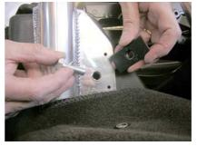
Drill 10 mm holes and fit the bolts as shown.
