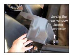
Carefully unclip the rear window heater connector from the trim panel. This will allow the complete removal of the trim panel.
