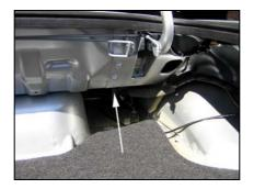
Removing these panels will provide the access needed to tighten the 4 mounting bolts used in securing the large flat mounting plate that is part of the roll bar assembly.
